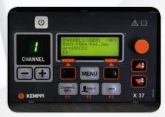
X 37 control panel of the FastMig X 450 power
