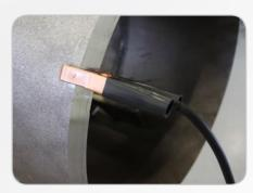
**Voltage sensing cable** measures the actual arc voltage during welding. This allows PipeRoot to optimise welding characteristics, which results in low-spatter filler material transfer and a stable welding arc.
