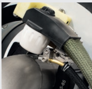
/ Wire feeding, torch bracket from 0 - 45° stepless swivelling
