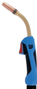
TBi 241 Classic Series 100% (10 min.) Mix: 270 A CO 2 : 300 A Ø 0.8-1.2 mm
