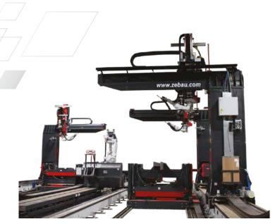
The **Steel Beam Assembler (SBA)** fully automated structural steel beam assembly and welding production line. The machine can fit and weld large amounts of steel accurately and efficiently.
