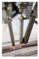
LSO combined to AC wave form, increase deposition rate up to 100%.
