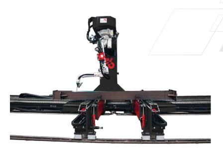
The **Steel Beam Welder (SBW)** is a robotic welding cell that can either weld out manually assembled beams or beams from an SBA, pre-assembled, and partially welded using the same work file generated for the SBA.
