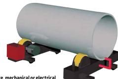
Anti-drift device, mechanical or electrical
