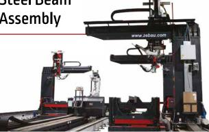
Beam welder & Clamping bench
