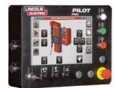
PILOT PRO Plus controller for a centralised management of the machine.
