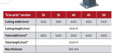
Traditional railways: R = additional rail of 1.5 m or 3 m / Useful travel maxi = 32 m Linear railways (option): R = additional rail of 2 m or 3 m / Useful travel maxi = 24 m
